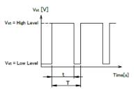
PWM Duty means that a ratio of high level time (t)/PWM Input Pulse(T).
